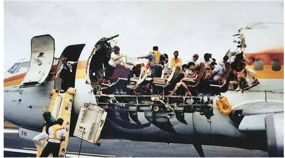
1988: Aloha Airlines Flight 243 Fatigue-cracking in lap-joint
