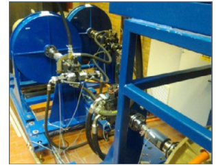
The hybrid hydrostatic drivetrain setup.
