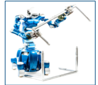
DLR's humanoid robot Agile Justin autonomously performing a complex construction task.
